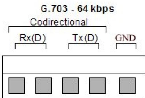
**Figure 3: ECMA 253 interface converter-terminal block connections**
