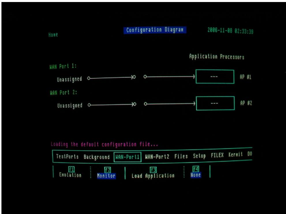
When the diagnostic and self test procedures are completed successfully, the PT502 should display the following screen, showing two WAN ports (Unassigned) and two Application Processors (Unloaded).
