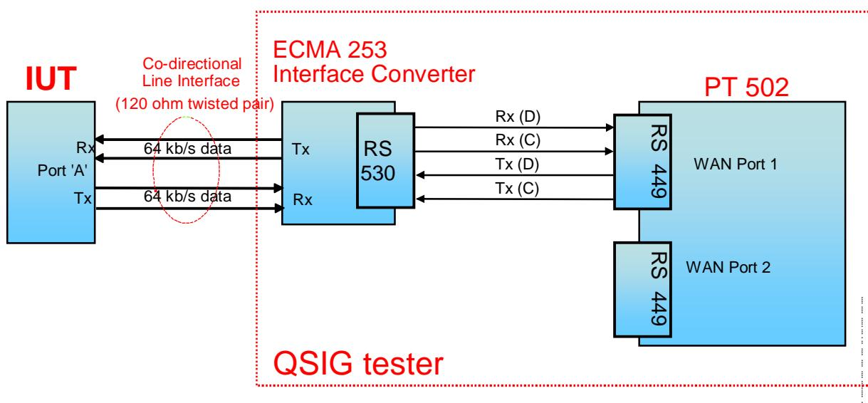
**Figure 1: Physical configuration for Conformance mono port test phases**
