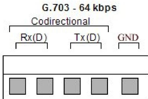
**Figure 8: ECMA 253 interface converter-terminal block connections**
