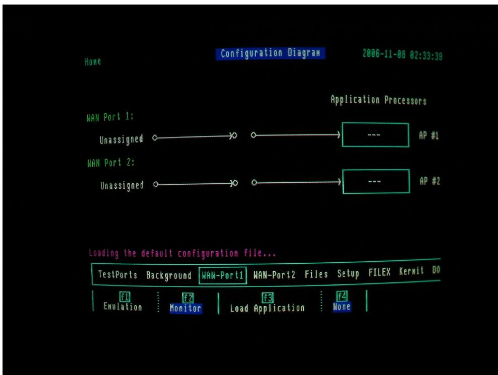
When the diagnostic and self test procedures are complete successfully, the PT502 should display the following screen, showing two WAN ports (Unassigned) and two Application Processors (Unloaded).
