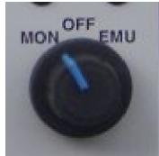
**Figure 9: ECMA 253 interface converter-Rotary switch configuration for Monitor**
