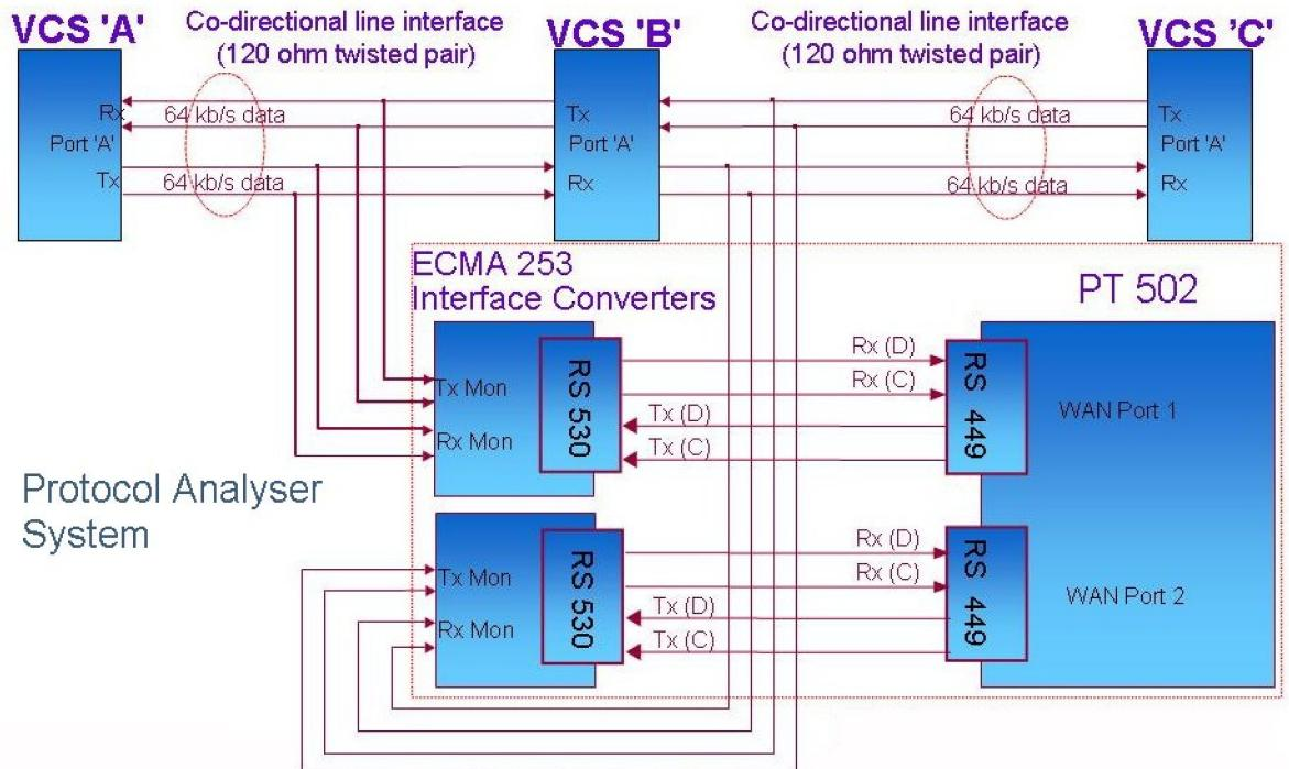
**Figure 7: Physical configuration for Monitoring dual links for transit interoperability**
