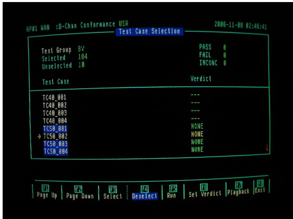
In order to select a Test Case that is not automatically selected by the PICS, it is necessary to return to the PICS statement and change the (S)election from RESTRICTED to UNRESTRICTED. In total there should be 310 test cases selected for the layer 2 test suite.
