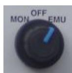
**Figure 5: ECMA 253 interface converter- Rotary switch configuration for Emulation**
