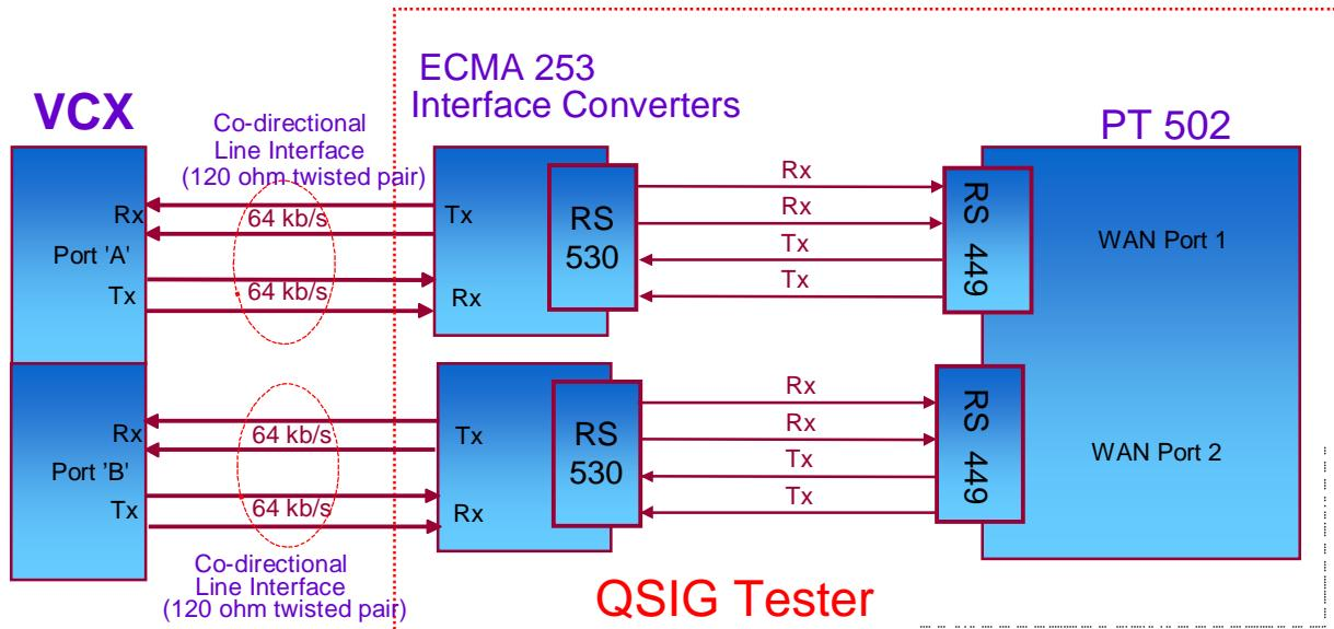
**Figure 2: Physical configuration for Conformance transit test phases**
